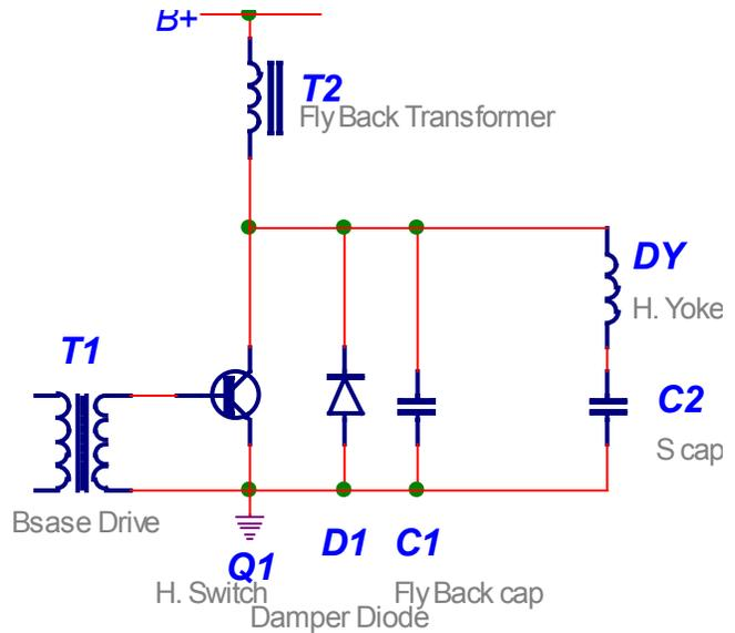
The voltage across the Q1 is a half sinusoid pulse during the flyback or retrace period and close to zero at all other times. It is not possible or safe to observe this point on an oscilloscope without a proper high frequency high voltage probe. Normally use a 100:1 probe suitable for 2,000V peak. The probe must have been high frequency calibrated recently.
