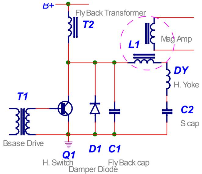
The large yoke current passes through a small number of turns of heavy wire. The flux from the yoke current makes a loop with an air gap in it. These two factors will give this coil little inductance and very high current handling ability. The flux density is far from saturation.
