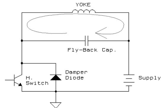
Time 4 represents the left hand half of the picture. Yoke current is negative and ramping down. The beam moves from the left to the center of the picture.
