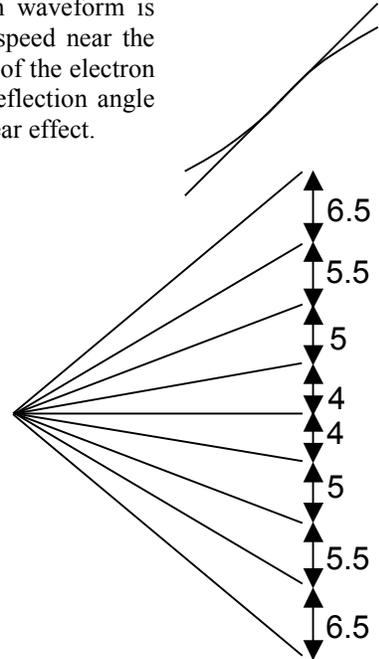
The S-cap value is very dependant on the scan rate. For multiscan monitors, S-caps must be selected for each scan range. These are only approximate corrections but good enough for most purposes. MOSFETs or relays switch in the correct S-cap for each range of scanning frequencies.
