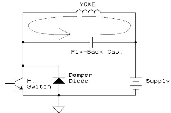
During time 3 the energy on the capacitor flows back into the yoke. The voltage on the flyback capacitor decreases while the current in the yoke builds until there is no voltage on the capacitor. By the end of time 3 the yoke current is at its maximum amount but in the negative direction. The beam is quickly deflected from the center to the left edge.
