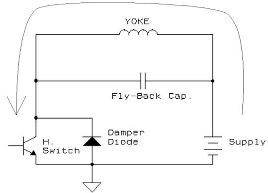
For time 2 the transistor is turned off. Energy transfers from the yoke to the flyback capacitor. At the end of time two all the energy from the yoke is placed on the flyback capacitor. There is zero current in the yoke and a large voltage on the capacitor. The beam is quickly moved from the right edge back to the middle of the picture.
