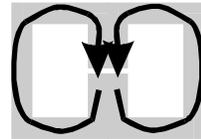
The control current passes through many turns of very small wire. The flux path does not have an air gap. The resulting coil will have high inductance and can be easily saturated by D.C. current. The outer legs of the transformer are saturated (in whole or in part) by the control current. Saturation in the outer legs causes a reduction in inductance in both coils.
