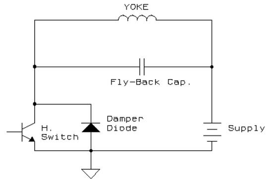
For time 1 the transistor is turned on. Current ramps up in the yoke. The beam is moved from the center of the picture to the right edge. Energy is stored on the inductance of the yoke.
